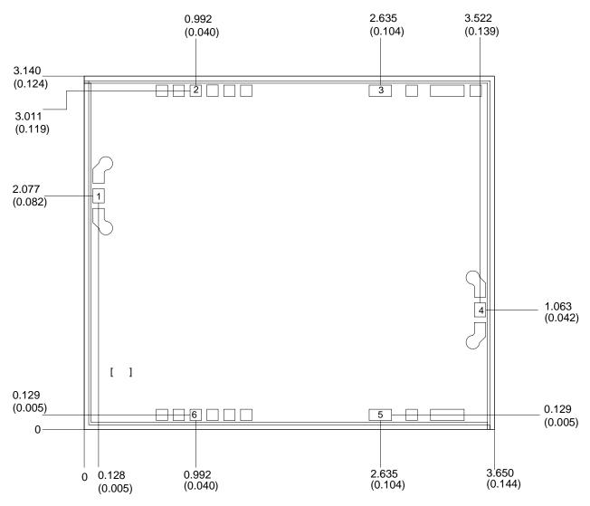
Units: Millimeters (inches) Thickness: 0.100 (0.004)
